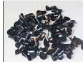
Chip samples produced with KRUZ-drill
